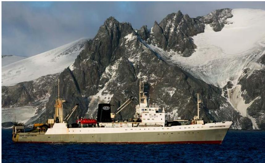
The F/V " More Sodruzhestva" trawler carries out the Antarctic krill catch and processing independently. The vessel is equipped with fishing gear, production halls, laboratory, freezer and cold storage. Food safety management system ISO 22000 have been implemented in production.
